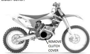
Remove the OEM clutch parts named in the following diagram down to the center hub. Leave the thrust washer installed in the basket.
