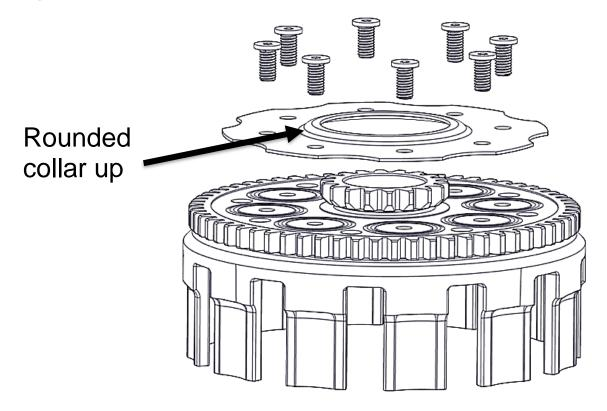
3. Tighten to **80 in-lb (9 N-m)** in a crisscross pattern to compress the assembly evenly.
