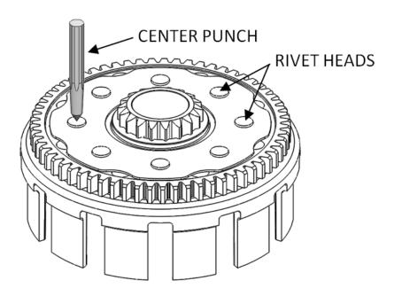
5.Use the supplied drill bit to drill out the heads of all the rivets. Set your drill to 300-400 RPM and use proper cutting fluid or oil for best results.
