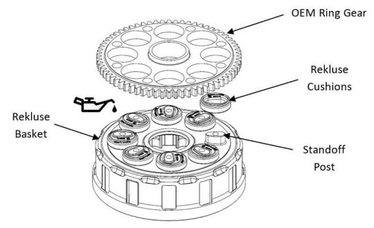
2. Install the Rekluse backing plate, then apply the supplied Loctite 262 to each of the M6 screws before threading them into the clutch basket assembly.
