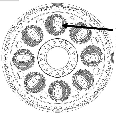
Starting from the top install dampers with the thick side of the damper to left of the standoff
