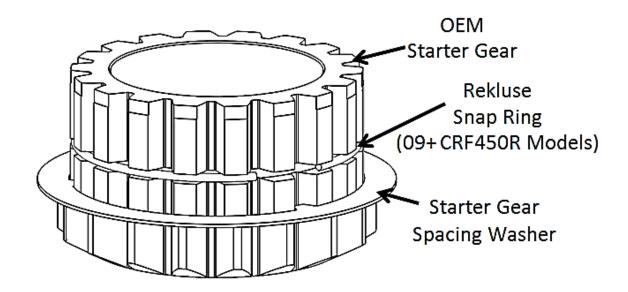
2. Place the Rekluse basket in a preheated oven at 400°F (200°C) for 15 minutes, making sure there is no oil on the basket. Place the starter gear, with the Rekluse supplied snap ring installed (09+ models only), in the freezer for the same duration.
