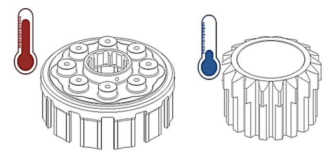
3. After 15 minutes, use oven mitts to remove the basket from the oven, then remove the starter gear from the freezer.
