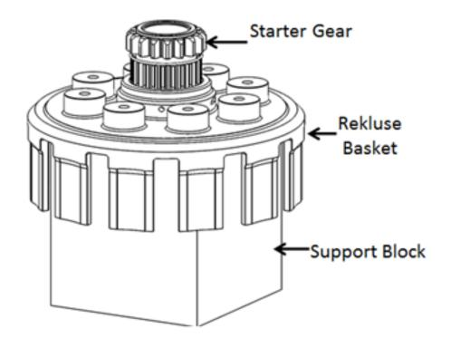
6. Once the basket has cooled, add some engine oil to the damper cushions and install one per standoff post.
