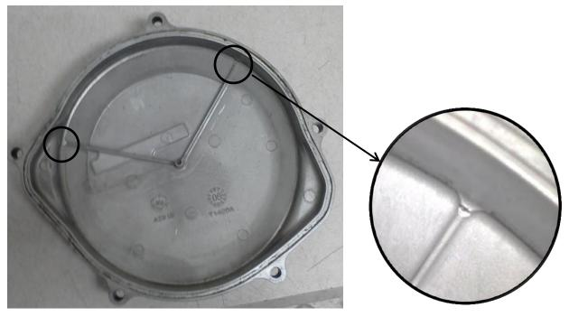
Use a file or small grinder to shave the ends of these ribs and reduce them to flush with the surfaces of the clutch cover.
