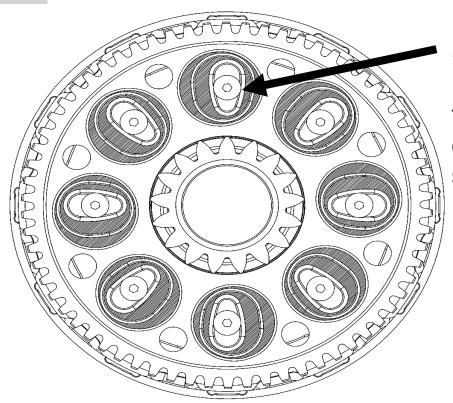
Starting from the top install dampers with the thick side of the damper to left of the standoff
