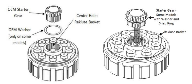
5. If the fit seems too tight due to the constraints of the snap ring, a shop press or vice may be needed to fully press in the gear. Support the basket (such as using a block of wood) when pressing in the starter gear. Pressing the gear in while the tangs are resting on a hard surface may damage the basket.
