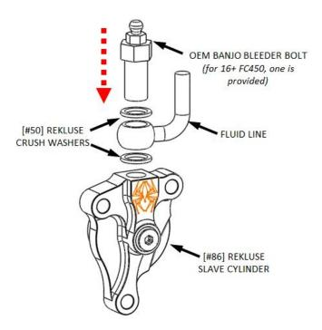
**NOTE:** Performed quickly, this method retains the fluid inside the line and makes the final bleeding step much easier.
