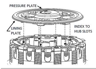
**20.** Install the OEM slider ring on the pressure plate with the "top" marking facing up. (The top side is rounded and the bottom edge is sharp.)
