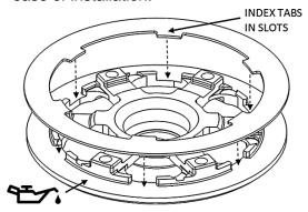
**19.** Install the pressure plate subassembly.
