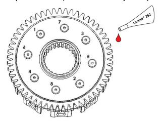
14. Using a hammer and center punch, peen the ends of the screws where they come through the bottom-inside of the clutch basket. Be sure to peen the screws. DO NOT peen the aluminum basket.
