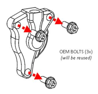
25. Mount the Rekluse slave cylinder to the engine using the OEM bolts.
