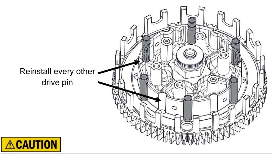
If pins are not in the correct slot, they may not be fully retained and could cause damage to the clutch engine. The pins should be covered during installation of the pressure plate if in the correct location.
