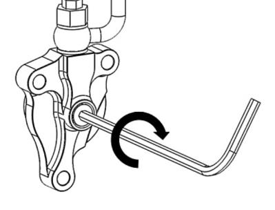
2.Once you have found the starting point, turn the adjuster clockwise 1 full turn plus 5 marks (or "1+5"). **This is NOT your final setting**, but it is a good reference point for using Free Play Gain to find the correct setting.
