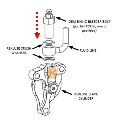
**NOTE:** A quick transfer of the fluid line will result in less bleeding in the following steps.
