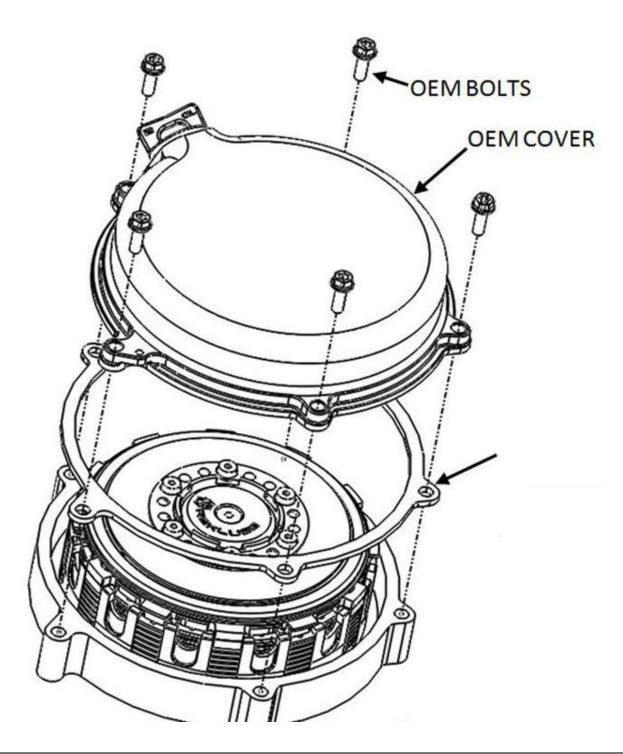
NOTE: If installing a Rekluse clutch cover, the spacing gasket is not needed.
