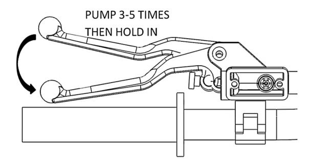
30. Using an 8mm wrench, open the bleed port. Air and fluid should come out of the bleed tube. Tighten the bleed port.
