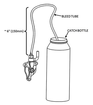
29. Pump the clutch lever 3-5 times then hold it against the bar/grip.
