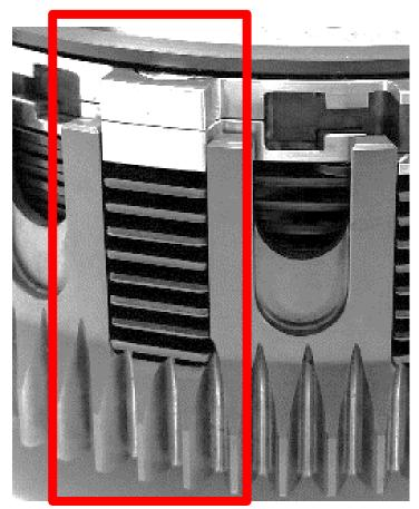
entire clutch pack, including the EXP disk, be installed into the MAIN (deeper) basket slots. Do not use the "half slots."
