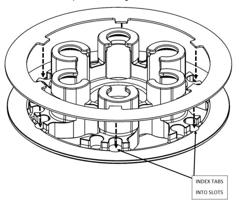
11. Install this pressure plate / lining plate combo, keeping the lining plate against the pressure plate. Hold the pressure plate against the clutch pack until it is bolted down in the later steps.
