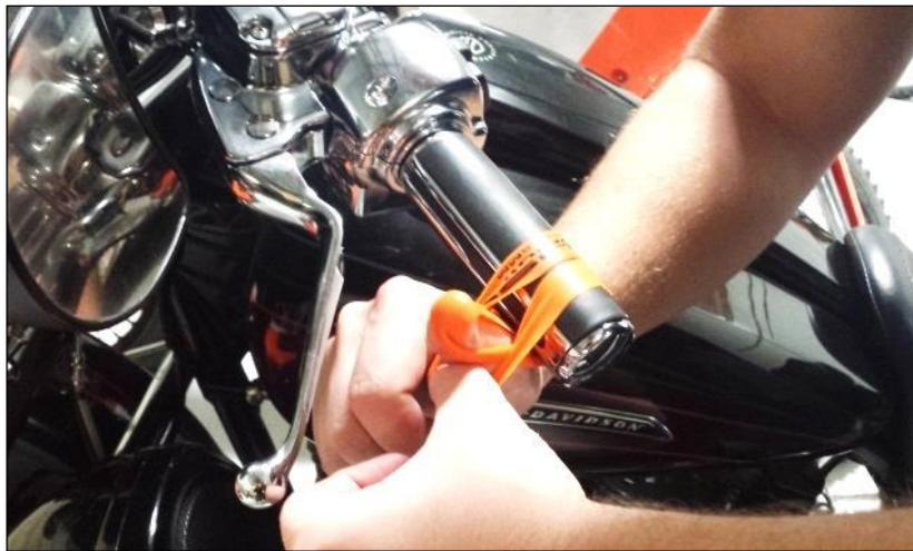
d) Pull the band through the loop, then attach it to the outside end of the clutch lever. This will take up the initial free play (slack) and put the lever in a position to detect the Free Play Gain.
