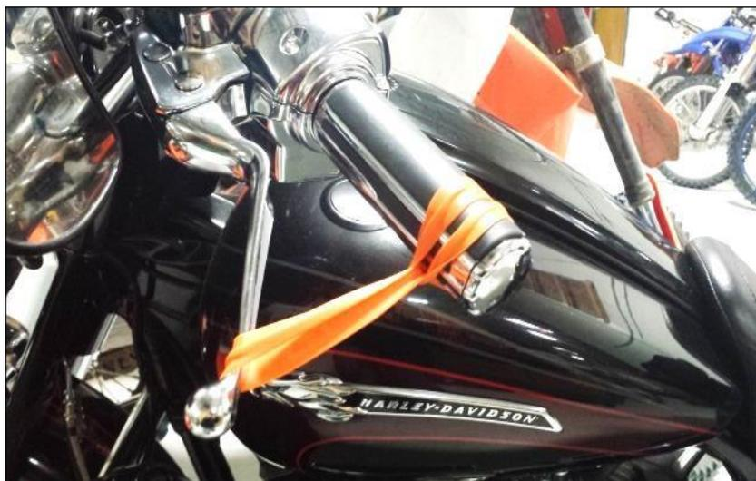
e) While still in **NEUTRAL**, quickly rev the engine between 3,000-5,000 RPM (1/4 to 1/2 throttle), then let it return to idle. Notice the movement in the clutch lever when the engine is revved. This is your Free Play Gain.
