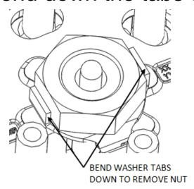
6. remove the center clutch nut with an impact wrench or breaker bar, and a 27 mm socket.
