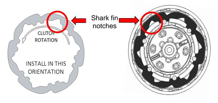
Be sure that the drive pins are seated in the notches and not in the bigger sections. ALL the TEC plates must be aligned in the drive pins notches or damage may occur. The plates will not move when installed correctly.
