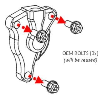
Mount the Rekluse slave cylinder to the engine using the OE bolts.
