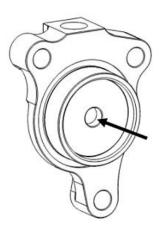
3. Pour the recommended clutch fluid into the slave cylinder port.
