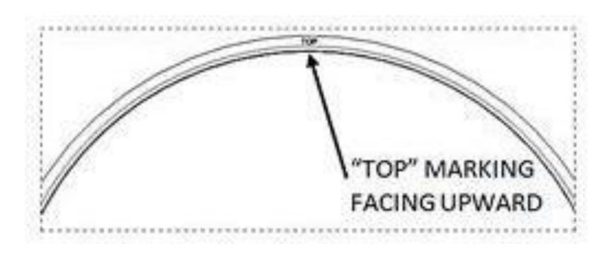
5. Place the OE Belleville spring onto the slider ring, with the rounded dome side facing up.
