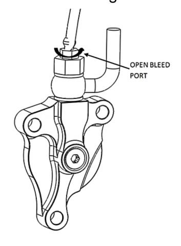
11. Slowly release the clutch lever and check the fluid level in the clutch master cylinder.
