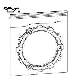
2. Install a steel TEC drive plate by first aligning the drive pin notches in the plate with the drive pins on the hub.
