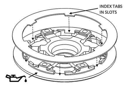
3. Install the pressure plate subassembly by lining up the index tabs on the pressure plate with the slots in the hub.
