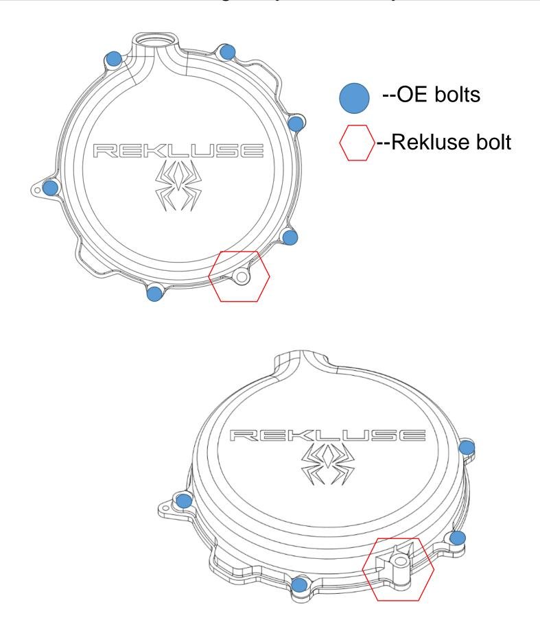
10. Install the Rekluse clutch cover by lightly tightening the cover bolts in a star pattern. Tighten bolts in small increments before torquing the cover bolts to OE specifications. If your bike has an oil plug, transfer the OE oil plug to the new Rekluse clutch cover.
