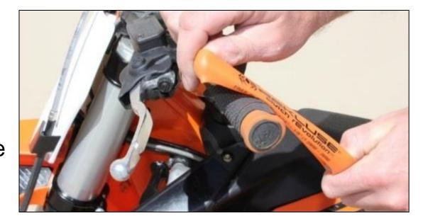
c) While holding the top end of the rubber band against the handlebar, stretch the band downward, then loop it through itself.
