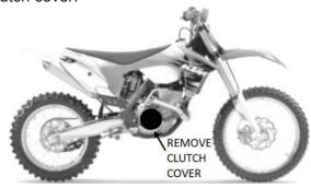
Remove the OEM parts named in the following diagram.
