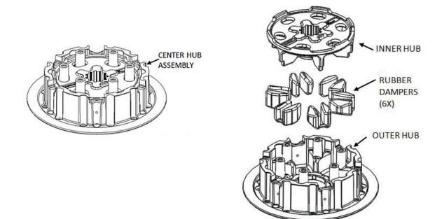
Over time, the rubber dampers will shrink due to heat and use. When this shrinkage occurs, the rotating action between the two hubs becomes loose or sloppy. This can cause hammering between the clutch parts which will reduce the life of the clutch.
