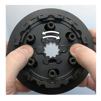
**7.** Remove the 6 rubber dampers from the center hub assembly.
