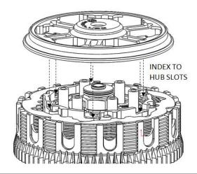
**16.** Install the OEM slider ring and Belleville spring.
