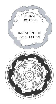
**13.** Install the rest of the clutch pack, noting the number and order of plates below.
