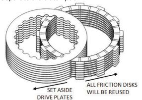
Inspect the friction disks for signs of heat or wear. Replace if they are burnt or worn.
