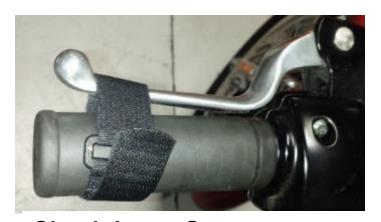
Clutch Lever Strap: to prevent unwanted launching.
