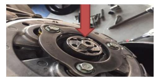
**Incorrect** – adjuster protruding out of adjuster assembly
