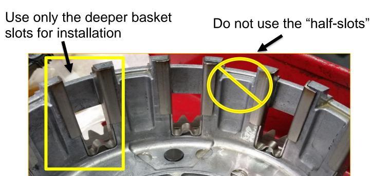
When assembling the clutch pack, it is important to line up the alignment notches on the friction disk tabs. *Correct alignment is critical for optimal performance*
