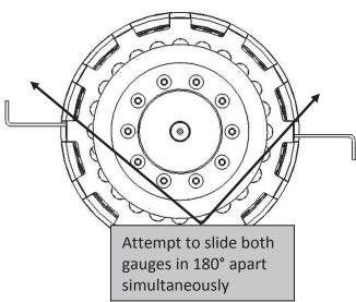
33. If the wire gauges slide in *smoothly*, the clutch pack needs adjustment. Swap the thick Rekluse adjustment drive plate for the top drive plate. Repeat step 32.
