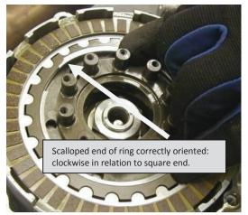
Threading retaining ring into groove
