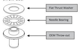
**NOTE:** RMZ250 bearing has rollers on only one side. Rollers MUST face down onto throw-out.
