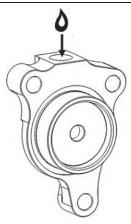
d. Turn the adjuster screw clockwise until it bottoms, keeping the fluid topped off as you go.
