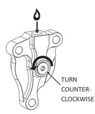
f. Compress the piston until it bottoms out. Repeat steps  $\mathbf{c}$ . –  $\mathbf{f}$ . until there is no longer air escaping from the top port when the piston is compressed.
