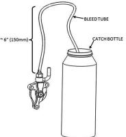
**37.** Pump the clutch lever 3-5 times then hold it against the bar/grip. Top off the fluid.
