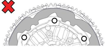
**Note:** ALL the TEC plates must be aligned in the drive pins notches or damage may occur. The plates will not move if installed correctly.
