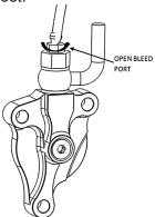
**39.** Slowly release the clutch lever and check the fluid level in the clutch master cylinder. Fill if necessary.
