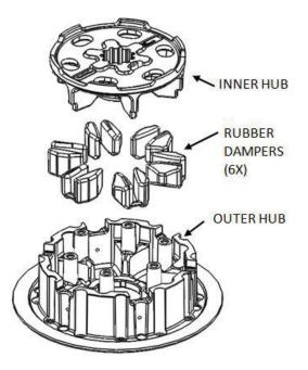
Over time, the rubber dampers will shrink due to heat and use. When this shrinkage occurs, the rotating action between the two hubs becomes loose or sloppy. This can cause hammering between the clutch parts which will reduce the life of the clutch.
