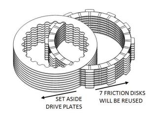
Inspect the friction disks for signs of heat or wear. Replace if they are burnt or worn with **KTM Part #: 59032011100**.
