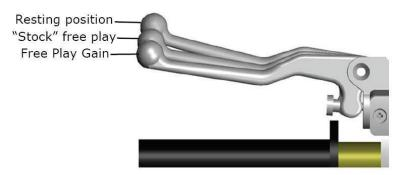
**Optimal Free Play Gain yields 1/8" (3mm)** of clutch lever movement, measured at the end of the lever. This measurement at the lever correlates to achieving the ideal installed gap.
