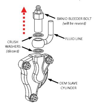
**29.** Next, attach this fluid line to the Rekluse Adjustable Slave Cylinder [#86] using the OEM Banjo Bleeder Bolt and the provided crush washers [#50]. Snug the banjo bolt with the unit in your hand. You will torque it to spec once installed on the bike.
