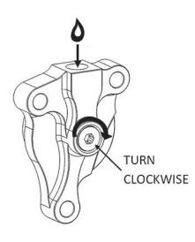
e. Turn the adjuster screw back to the initial position with the top O-ring visible.
