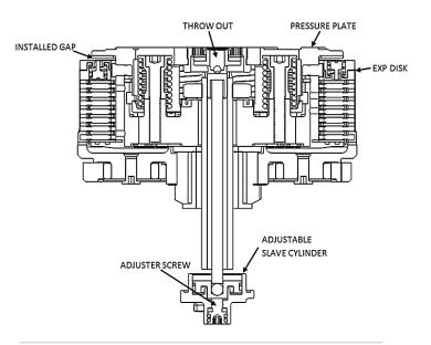
**42.** Using the long end of a 4mm Allen key, turn the adjuster screw clockwise until it stops under moderate pressure. You are trying to feel for the point at which the throw-out will start to lift the pressure plate. This is the "starting point."
