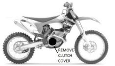
**NOTE**: Take note of each OEM clutch cover bolts specific location as length can vary between them. Failure to replace these bolts in the proper location after clutch installation can result in damage to your motorcycle.
