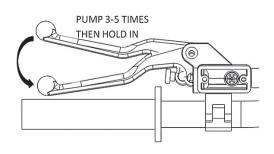
**38.** Using an 8mm wrench, open the bleed port while continuing to hold on the clutch lever at the handlebar. Air and fluid may flow from the bleed tube. Tighten the bleed port when pressure is lost.
