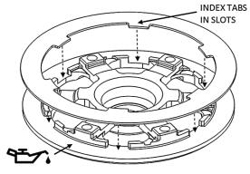
**19.** Install the pressure plate subassembly.
