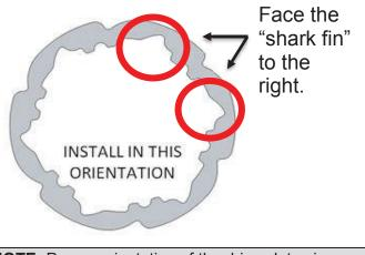
**NOTE:** Proper orientation of the drive plates is *critical* for optimal clutch performance. If you install them backwards, the clutch will still function but will lack proper modulation performance.
