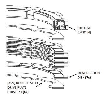
**16.** Install the EXP disk on top of the last steel plate. Make sure that the EXP disk is seated in the same slots as the clutch pack.
