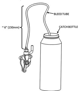
**25.** Pump the clutch lever 3-5 times then hold it against the bar/grip.
