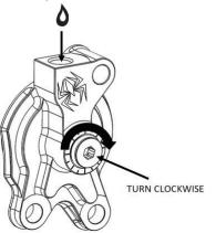
e. Turn the adjuster screw back to the initial position while compressing the piston until it bottoms out. Repeat this process until there is no longer air escaping from the top port when the piston is compressed.
