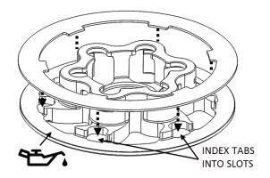
**14.** Install this pressure plate subassembly.
