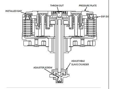
29. Using the long end of a 4mm Allen key, turn the adjuster screw clockwise until it stops under moderate pressure. You are trying to feel for the point at which the throwout will start to lift the pressure plate. This is the "starting point".
