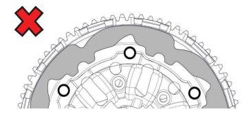
**Note:** ALL the TEC plates must be aligned in the drive pins notches or damage may occur. The plates will not move if installed correctly.
