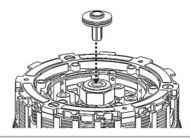
**13.** Place the Steel Lining Plate [#16] onto the Rekluse Pressure Plate [#5]. Adding an oil film between them will help them stick together.
