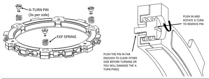
**CAUTION:** If you disassemble the EXP, bearing pads may fall out or be stuck to the ramp surfaces of the EXP bases. Take care to ensure all pads are correctly placed into wedge pockets using gentle pressure to avoid damage to the pad surfaces before reassembling the EXP. Properly seated pads will be secured in place once the EXP is reassembled. Operating the clutch without the pads in place will cause part damage or failure.
