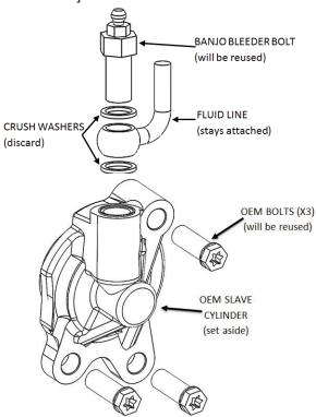
**19.** On a workbench (still away from the engine), bleed the Rekluse slave cylinder by this procedure:
