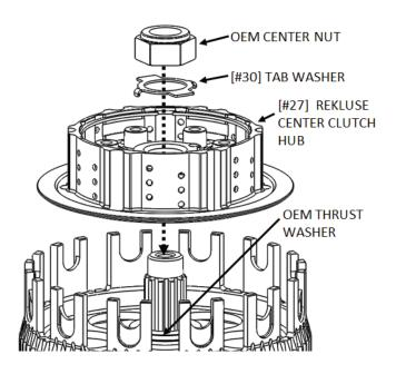
Torque the nut to 50 ft-lb (68 N-m), then bend up both tabs of the tab washer using channellock pliers.
