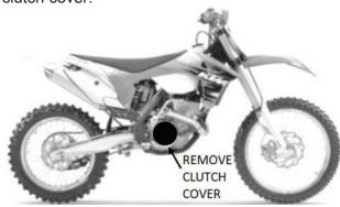
2. Remove the OEM clutch parts named in the following diagram including the center hub. Leave the thrust washer installed in the basket.
