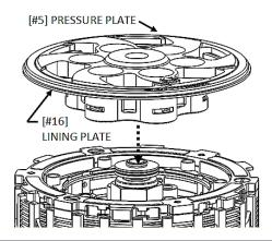
**15.** Install the Rekluse pressure plate springs and torque the pressure plate bolts.
