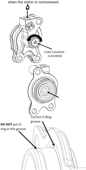
**NOTE:** When compressing the piston, fluid can shoot out from the slave cylinder port. Be sure to wear eye protection.
