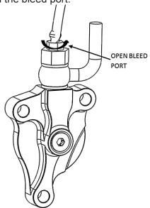
**27.** Slowly release the clutch lever and check the fluid level in the clutch master cylinder.
