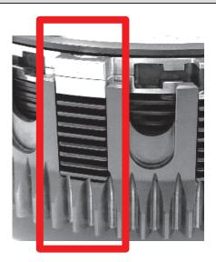
7. Seat 6 of the OEM drive pins into the hub.
