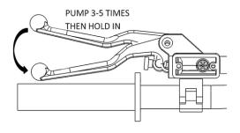
**26.** Using an 8mm wrench, open the bleed port. Air and fluid should come out of the bleed tube. Tighten the bleed port.
