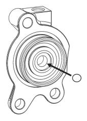
**21.** Install the Rekluse slave cylinder on the bike using these parts, ending with the banjo bolt.
