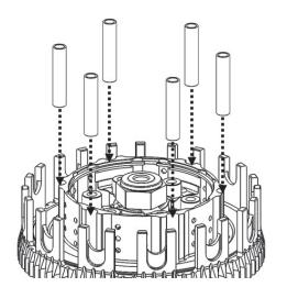
8. Hold a TEC drive plate so that the "shark fin" notches face toward the right. *All the drive plates will follow this orientation.*
