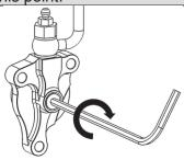
**30.** Once you have found the starting point, turn the adjuster clockwise 1 full turn plus 5 marks (or "1+5"). **This is NOT your final setting**, but it is a good reference point for using free play gain to find the correct setting.
