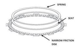
• If judder spring and seat are installed, assemble the clutch following the graphic on the next page. .
