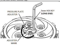
10. At this point, make a note of where the mark on the adjuster aligns with the tick marks on the pressure plate. This is your **starting point**.
