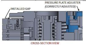
Insert the long end of a 5-mm hex key into one of the two hex holes in the pressure plate adjuster. By hand, gently thread the pressure plate adjuster inward until it comes to a stop against the center clutch nut.
