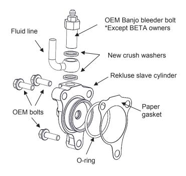
**NOTE:** Only some models have a paper gasket and/or O-ring seal. Reuse the OEM gasket and seal if not supplied.
