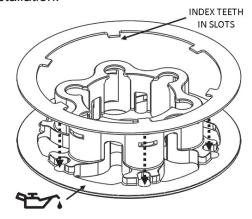
**12.** Install this pressure plate subassembly.
