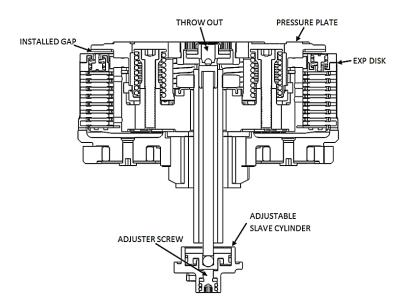
28. Using the long end of a 4mm Allen key, turn the adjuster screw clockwise until it stops under moderate pressure. You are trying to feel for the point at which the throw-out will start to lift the pressure plate. This is the "starting point".
