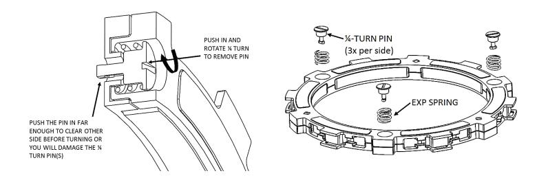
**CAUTION:** If you disassemble the EXP, bearing pads may fall out or be stuck to the ramp surfaces of the EXP bases. Take care to ensure all pads are correctly placed into wedge pockets using gentle pressure to avoid damage to the pad surfaces before reassembling the EXP. Properly seated pads will be secured in place once the EXP is reassembled. Operating the clutch without the pads in place will cause part damage or failure.
