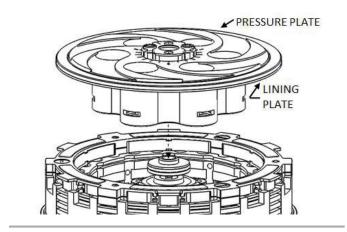
**13.** Install the pressure plate springs.
