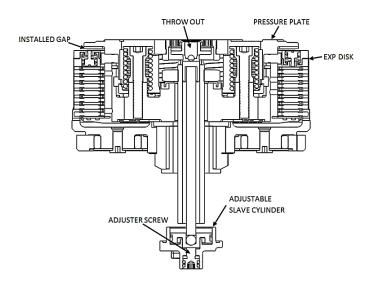
**35.** Using the long end of a 4mm Allen key, turn the adjuster screw clockwise until it stops under moderate pressure. You are trying to feel for the point at which the throw-out will start to lift the pressure plate. This is the "starting point".
