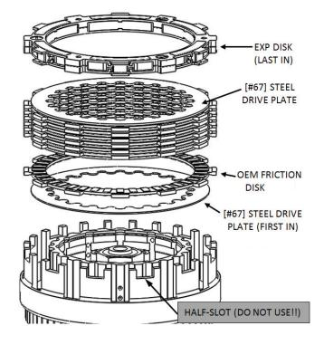
**9.** Install the included Rekluse throw-out assembly in the order shown in the following diagram on top of the stock throw-out rod.
