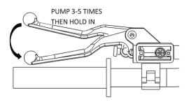
**31.** Using an 8mm wrench, open the bleed port. Air and fluid should come out of the bleed tube. Tighten the bleed port.
