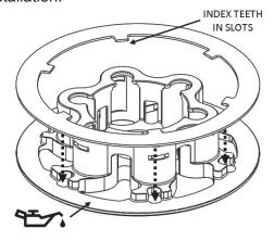
11. Install this pressure plate subassembly.
