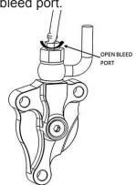
**32.** Slowly release the clutch lever and check the fluid level in the clutch master cylinder.
