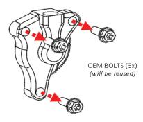
**21.** Mount the Rekluse slave cylinder to the engine by lightly threading the two shorter OE bolts on the left side until finger tight.
