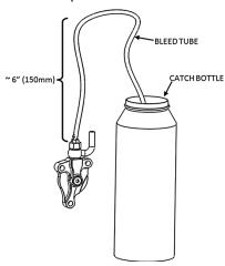
**30.** Pump the clutch lever 3-5 times then hold it against the bar/grip.
