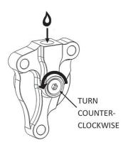
f. Compress the piston until it bottoms out. Repeat the process until there is no longer air escaping from the top port when the piston is compressed.
