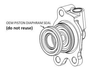
20. With the clutch fluid line attached to the Rekluse slave cylinder, remove the OE slave cylinder from the engine. Keep the OE bolts for reuse.
