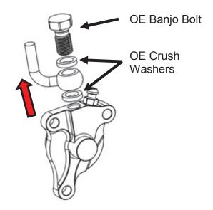
**18.** Attach the clutch fluid line to the Rekluse slave cylinder using the OE banjo bolt and the 2 new crush washers from Rekluse. Make sure the banjo fitting is between the 2 crush washers.
