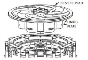
12. Install the pressure plate springs.
