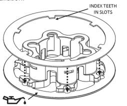
**11.** Install this pressure plate subassembly.
