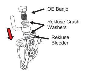
**19.** Tighten the banjo bolt with your hand until snug. (You will torque it to spec once installed on the bike.)
