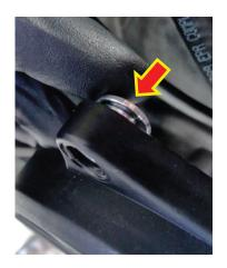
**24.** Reattach the chain guard to the slave cylinder using the longer OE screw.
