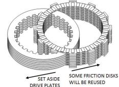
Inspect the friction disks for signs of heat or wear. Replace if they are burnt or worn. For most models, new friction disks can be purchased from Rekluse.
