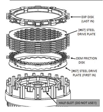
**9.** Install the included Rekluse throw-out assembly in the order shown in the following diagram on top of the stock throw-out rod.
