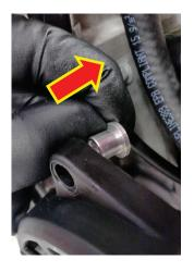
**23.** Insert the new Rekluse chain guard screw sleeve into the screw slot.
