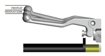
Optimal Free Play Gain yields **1/8" (3mm)** of clutch lever movement, measured at the end of the lever. This measurement at the lever correlates to achieving the ideal installed gap.
