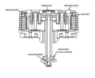
**35.** Using the long end of a 4mm Allen key, turn the adjuster screw clockwise until it stops under moderate pressure. You are trying to feel for the point at which the throw-out will start to lift the pressure plate. This is the "starting point".
