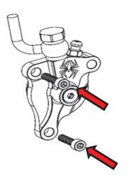
**22.** Remove the OE chain guard screw sleeve from the plastic chain guard by gently pushing it out the backside.
