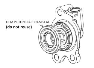
**20.** With the clutch fluid line attached to the Rekluse slave cylinder, remove the OE slave cylinder from the engine. Keep the OE bolts for reuse.
