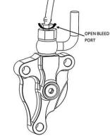
**32.** Slowly release the clutch lever and check the fluid level in the clutch master cylinder.
