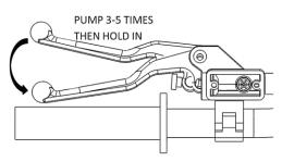
**31.** Using an 8mm wrench, open the bleed port. Air and fluid should come out of the bleed tube. Tighten the bleed port.
