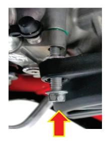
**NOTE:** The Rekluse screw sleeve is slightly taller than the OE screw sleeve. You will need to use the Rekluse screw sleeve to help ensure a good seal to the engine case.
