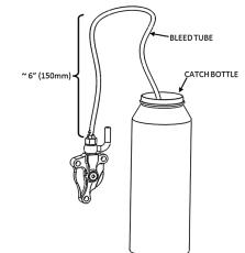
**30.** Pump the clutch lever 3-5 times then hold it against the bar/grip.
