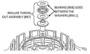
**NOTE**: If you are missing the top washer, it is probably stuck to the backside of your OEM pressure plate.
