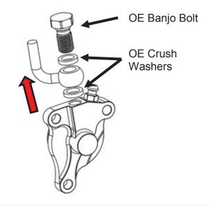
**18.** Attach the clutch fluid line to the Rekluse slave cylinder using the OE banjo bolt and the 2 new crush washers from Rekluse. Make sure the banjo fitting is between the 2 crush washers.
