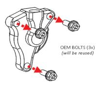
**21.** Mount the Rekluse slave cylinder to the engine by lightly threading the two shorter OE bolts on the left side until finger tight.
