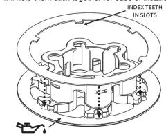
7. Install this pressure plate subassembly.
