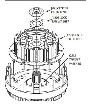
**NOTE**: If the OEM thrust washer is not in place, it is probably stuck to the backside of your OEM center clutch hub.
