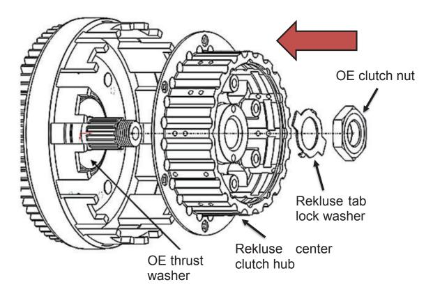
5. Using the socket and torque wrench, torque the center clutch nut to 50 ft-lb (68 N-m).
