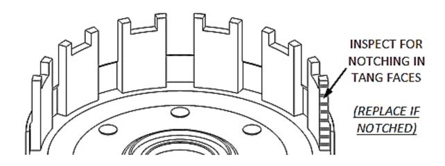
**Note:** If the basket is notched or worn, Rekluse recommends replacing it with a Rekluse Billet Clutch Basket (available for most models).
