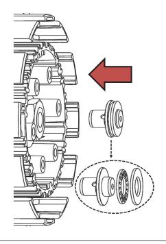
If the washer is missing: Check to see if it is stuck to the backside of the OE pressure plate
