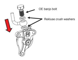
**NOTE:** A quick transfer of the fluid line will result in less bleeding in the following steps.
