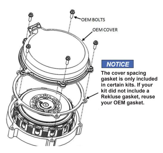
17. Install the clutch cover bolts in their proper OEM location. Lightly tighten the cover bolts in a star pattern. Torque the bolts in small increments before tightening all the bolts. Torque the cover bolts to OEM specification – **7.4** ft-lb (**10** N-m).
