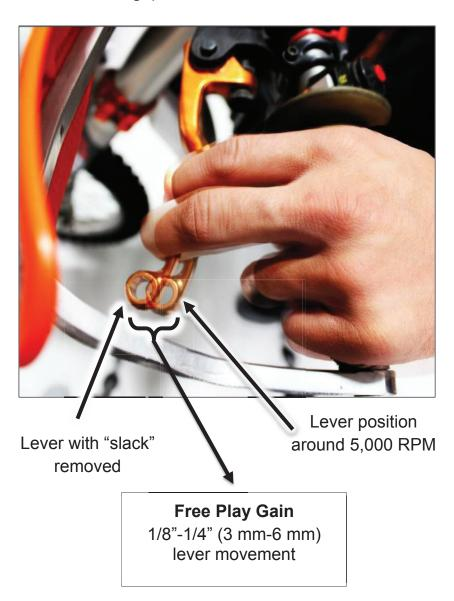
The following steps explain two ways to check Free Play Gain. One will use the rubber band that has been included in the clutch kit and one explains using your hand, which you will perform before every ride.
