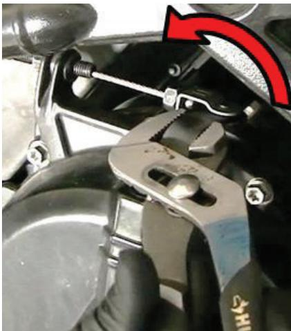
**NOTE:** After you complete the steps in the next section (setting and verifying the installed gap), the actuator arm will rest at nearly 90 degrees to the cable, as shown here.
