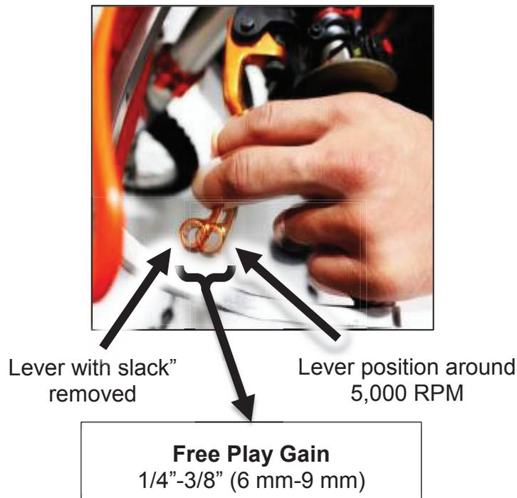
When the bike returns to idle, rest your hand across the clutch lever. Rev the engine again to 3,000-5,000 RPM so you can observe the movement while feeling for Free Play Gain with your hand.
