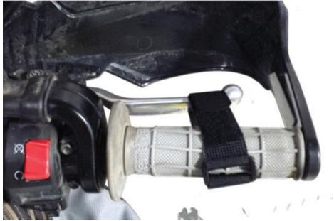
**Clutch Lever Strap:** to prevent unwanted launching.
