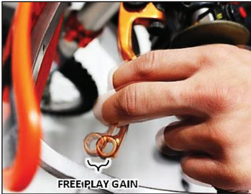
4. Now that the EXP is broken-in and the clutch is warm, re-check free play gain at your clutch lever and adjust if necessary. Your clutch pack will expand with heat, so final adjustments should be made when the bike is warm. Now you are ready to ride!
