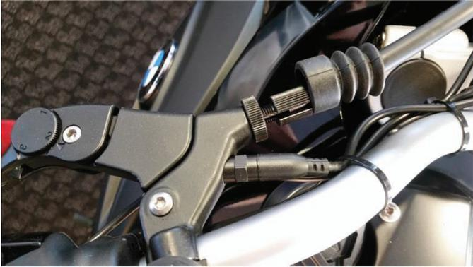
11. Use channel-lock pliers to reattach the clutch cable to the actuator arm. The cable should be tight at this point.
