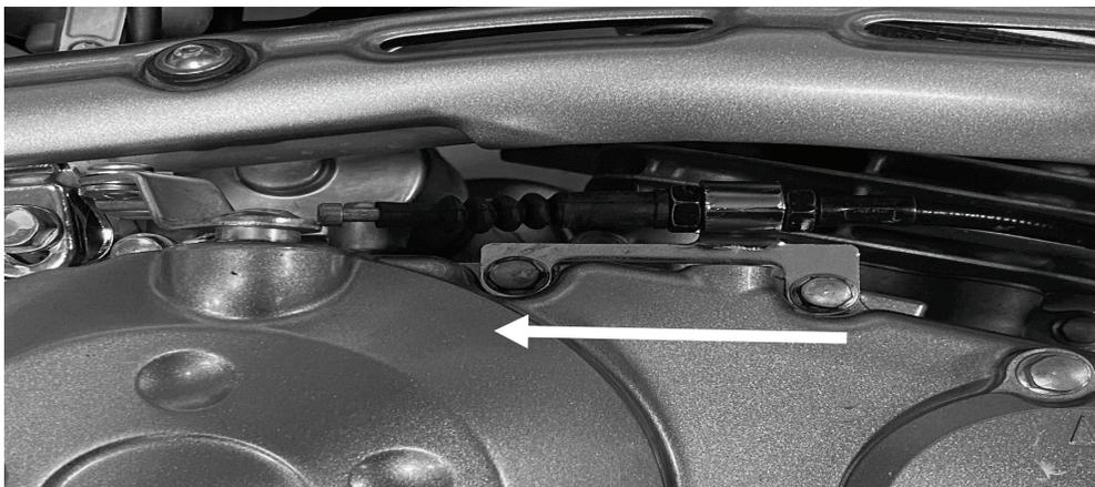
30. Attach the clutch cable to the actuator arm. Using a crescent wrench to move the actuator arm towards the cable makes attaching the cable easier.
