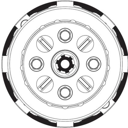
24. Install the center clutch bolt. Torque to 48 ft-lb (65 N-m).
