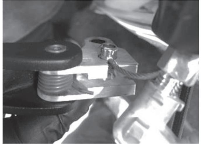
4. Using an end wrench or T handle install the Rekluse clutch lever. Tighten your perch bolt to OEM specification.
