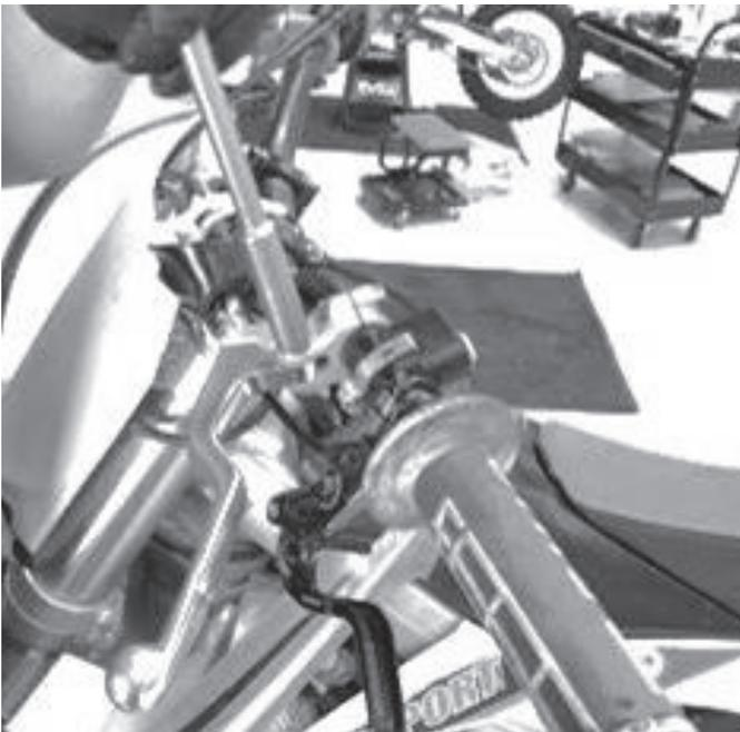
3. Index the cable into the backside of the Rekluse adjustable reach lever.
