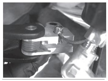
**4.** Using an end wrench or T handle install the Rekluse clutch lever. Tighten your perch bolt to OEM specification.
