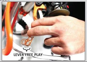
For Kawasaki & Suzuki Auto-Clutches (Rekluse CoreEXP): Follow the instructions in your CoreEXP User's Guide to properly set the installed gap by checking lever free play gain.
