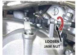
**NOTE:** The clutch cable does not have to be removed from the clutch cover to enable access to the clutch. See the next steps for the procedure to tilt the cover out of the way.
