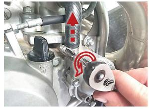
**1g.** Both the water pump housing and the coolant-out hose can be moved out of the way of the clutch cover by gently tucking them between the engine and the exhaust
