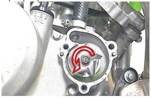
1f. Using a 6mm socket, loosen the hose clamp on the hose that goes from the cylinder to the clutch cover (the coolant-out hose). Then remove the hose end from the clutch cover.
