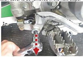
**5.** Remove all of the clutch cover bolts, and then lift the clutch cover free of the kick-start and water pump shafts.
