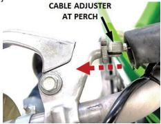
**1i.** At the threaded adjuster, use a 10mm endwrench to loosen the jam nuts — removing tension from the clutch cable to the position of maximum cable/lever slack.
