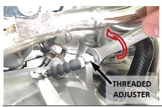
**NOTE:** "Lever Free Play" is essentially the "slack" in the clutch cable system felt at the lever before it starts actuating the clutch. Applying a light finger pressure will take up this slack.
