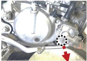
**1c.** Making sure that the engine/coolant is not hot, twist open the radiator cap to help evacuate all the coolant from the system into the container.
