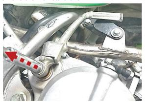
4. Remove the brake pedal pivot bolt using an 8mm Allen. Then, uncouple the spring from the pedal and move the pedal out of the way. This will provide access and clearance for the clutch cover to be removed in the next steps.
