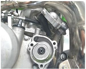
**1h.** At the lever perch, remove all tension from the clutch cable by twisting the perch adjuster clockwise until it bottoms out.
