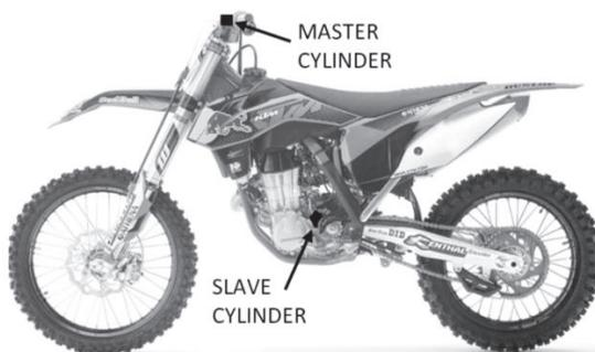
1. With the bike resting on its center stand or leaning on its kickstand, use a 13mm box-end wrench to remove the banjo bolt from the OEM slave cylinder. Be ready to catch the fluid that drains out of the line.
