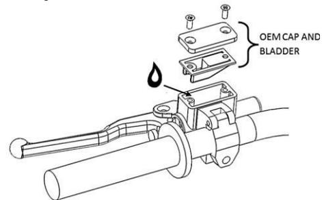
7. Fill the provided syringe with clutch fluid.
