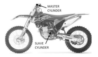
2.On the left side of the bike, while leaving the OE slave cylinder intact on the engine, remove the banjo bolt and the 2 OE crush washers from the OE slave cylinder. Discard the OE crush washers.
