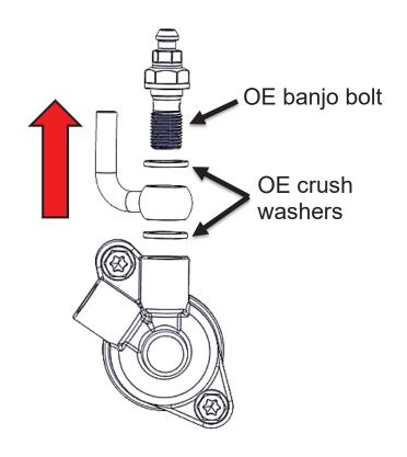
Pg. 6 Doc ID: 194-102A Doc Rev: 100818 3. Attach the clutch fluid line to the Rekluse slave cylinder using the OE banjo bolt and the 2 new Rekluse crush washers. *Make sure the fluid line is sandwiched between the 2 crush washers.*
