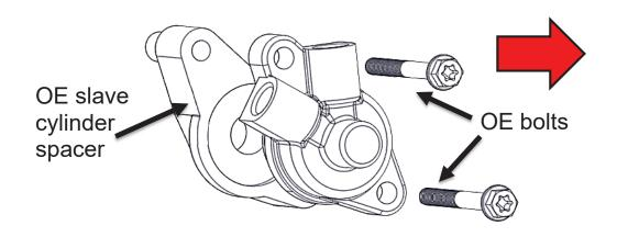
6. Mount the Rekluse slave cylinder to the engine using the OE slave cylinder spacer and OE bolts. Torque to OE specifications.
