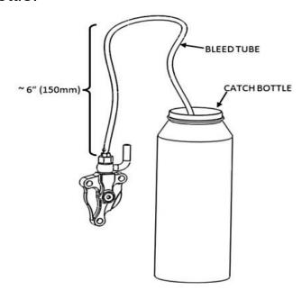
Pg. 8 Doc ID: 194-102A Doc Rev: 100818 2.On the handlebar, remove the cap and bladder from the clutch master cylinder. Adjust the reservoir so it is level with the ground.
