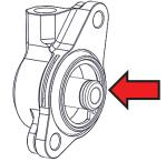
2. While holding the slave cylinder piston, pour the appropriate clutch fluid into the slave cylinder port until it is full.
