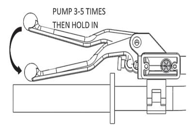
5. While still holding the clutch lever in, use a wrench to open the bleed port. Air and fluid should flow from the bleed tube into the catch bottle.
