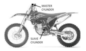
2.On the left side of the bike, while leaving the OE slave cylinder intact on the engine, remove the banjo bolt and the 2 OE crush washers (or the fluid line-in) from the OE slave cylinder (depending on your bike model). Discard the OE crush washers.
