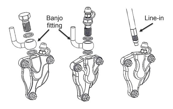
Pg. 8 Doc ID: 194-2400A Doc Rev: 042821 3. Attach the clutch fluid line to the Rekluse slave cylinder using the OE banjo bolt and the 2 new Rekluse crush washers (if applicable). Make sure the banjo fitting is sandwiched between the 2 crush washers.
