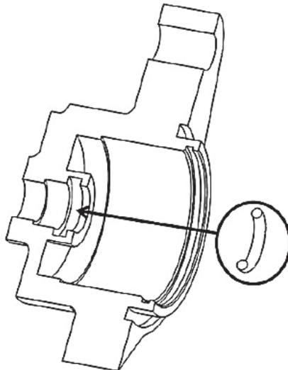
5. Using snap-ring pliers, remove the snap ring from the cylinder housing.
