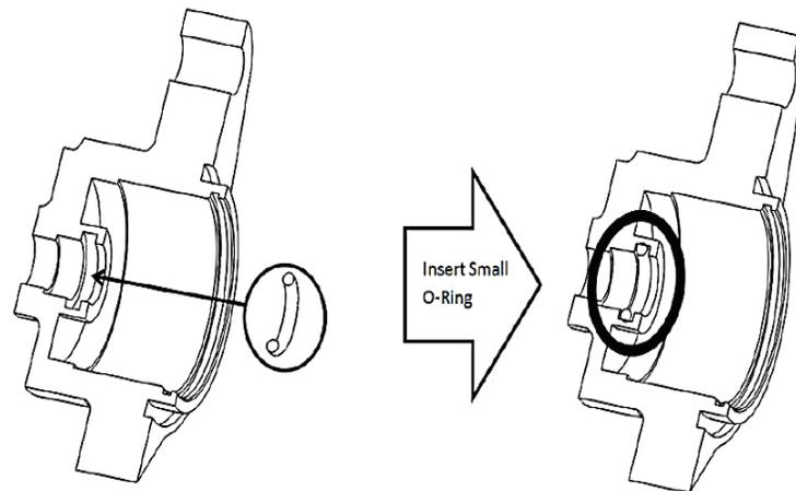
**For Newer Models:** Carefully install 2 new small O-ring seals into the grooves on the adjuster screw (these will always be the same color: either both brown or both black, depending on clutch fluid type). Then, reinstall the adjuster screw into the housing.
