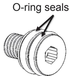
3. Carefully install the new medium-sized O-ring seals into the piston grooves.
