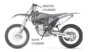
2. Using a 4 mm hex key, remove the adjuster screw from the slave cylinder housing by turning it **counterclockwise**. Catch any draining fluid in a suitable container, and dispose of it according to local regulations.
