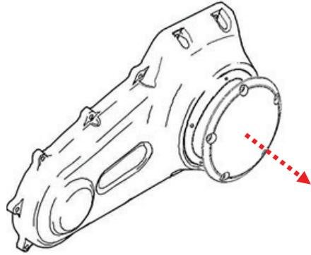
2. Remove the gasket or O-ring from the derby cover and inspect it for wear or damage. Replace if necessary.
