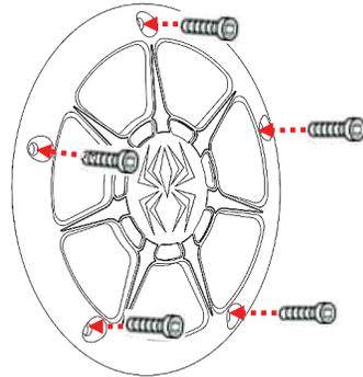
5. Lightly tighten the cover screws in small increments, then torque to **90-120 in-lbs (9.5-12.2 N-m)** per OE specifications.
