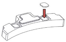
4. Use the flat part of a flat blade screwdriver or similar tool to press the Teflon pad into the wedge. You many need to turn the wedge around and press on the opposite side to get the pad to fully seat.
