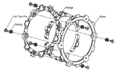
3. Inspect the EXP bases. Do not reinstall the wedges into worn bases. See the video at https://rekluse.com/support/videos for instructions on how to inspect the EXP disk.
