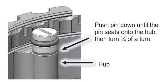
c. The spring will push the pin back up once it is released. The bottom groove is visible when the pin is locked.
