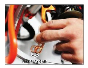
c) While still in **NEUTRAL**, continue to apply light pressure and quickly rev the engine between 5,000-7,000 RPM (1/2 to <sup>3</sup>/<sub>4</sub> throttle), then let it return to idle. Notice the movement in the clutch lever when the engine is revved. This is your Free Play Gain.
