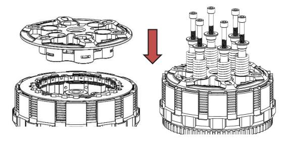
**Note:** Be sure to alternate springs if you are using two different color springs to keep even pressure on the clutch. Heavier springs are available for purchase from Rekluse for high horse-power applications.
