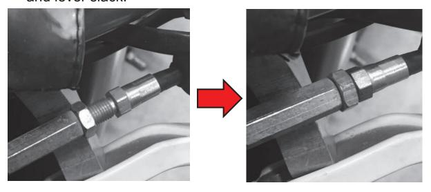
9. At the in-line cable adjuster, tighten the clutch cable tension to the point where there is no lever freeplay (the clutch lever is tight against its perch). At this point, there should be no cable slack.
