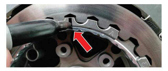
**Note:** It does not matter where you draw the mark as long as it is over one of the circle detents on the adjustment ring. You may need to wipe the oil off the adjustment ring and hub before marking the ring.
