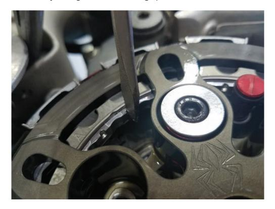
6. Once you find the starting point, remove the pressure plate by removing the pressure plate bolts, screw sleeves, and springs, then remove the pressure plate.
