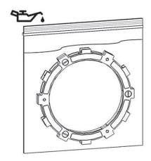
2. Install all the Rekluse basket sleeves into the basket slots. Make sure the bottom of the sleeve is facing down, and the sleeve tabs sit against the inside of the basket. (See the following pictures for reference.)
