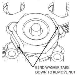
12. Remove the center clutch nut with an impact wrench or breaker bar, and socket. Set aside. The OE clutch nut will be reused.
