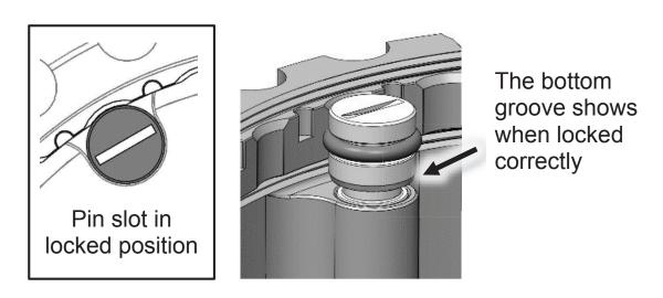
**Note:** The ring will move slightly when the pin is locked. This is normal.
