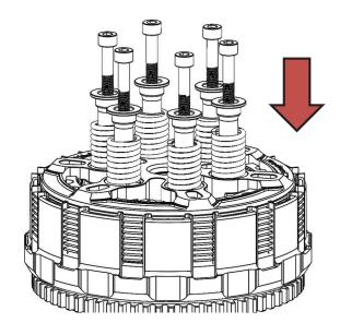
**Note:** Use all 6 springs to fully compress the judder spring for the proper initial adjustment. Tighten the bolts until snug. They will be removed in a later step.
