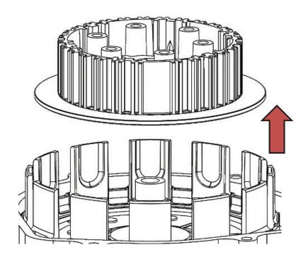
**Note:** Check that the OE thrust washer is still on the main shaft and not stuck to the bottom of the center hub assembly. The thrust washer must be installed, or clutch performance issues will result.
