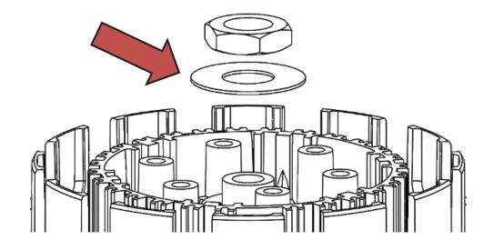
14. Remove the center hub from the clutch basket while leaving the underneath thrust washer on the main shaft.
