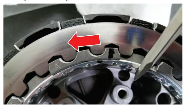
9. Start at the reference mark, then turn the adjustment ring **CLOCKWISE 2 circle detents** passed your mark on the hub.
