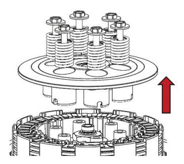
8. Remove the OE clutch pack, then set aside all the plates. Use a pick if necessary to help remove all the plates.
