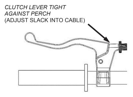
10. Expand the in-line cable adjuster housing 5 turns to lift pressure plate. This is not your final setting. It is your *starting point* for setting the installed gap. This will vary by bike.
