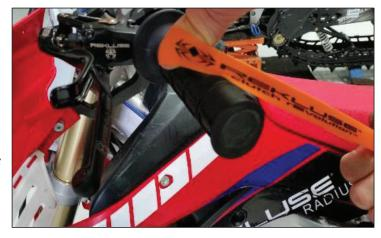
c) While holding the top end of the rubber band against the handlebar, stretch the band downward, then loop it through itself.
