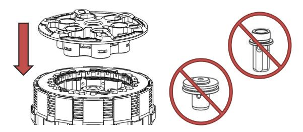
2. Insert the pressure plate springs and screw sleeves, then insert the pressure plate spring bolts into the screw sleeves.
