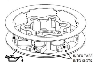
3. Install the pressure plate subassembly.
