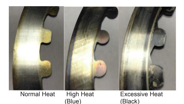
**Friction Disks** – Due to the dark color of the friction material, the friction disks will appear almost black as soon as they are put in oil. During inspection, look for glazing of the friction material. Glazing will appear shiny and feel like glass, even after oil is cleaned from the friction disk. Not all friction disks look the same and may look different than pictured.
