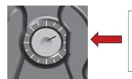
Use the tick marks on the cylinder and the etch mark on the screw to remember the starting point for adjusting the gap.
