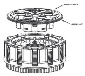
4. Place the pressure plate springs into the assembled clutch, then insert the screw sleeves into the springs. See the following chart for spring information.
