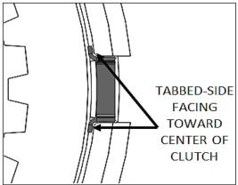
**Note:** When seated in the basket, the sleeves may stick slightly above or below flush with the top of the basket. This is normal.
