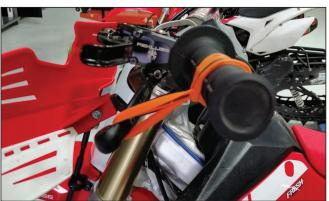
e) While still in **NEUTRAL**, quickly rev the engine between 5,000-7,000 RPM (1/2 to ¾ throttle), then let it return to idle. Notice the movement in the clutch lever when the engine is revved. This is your Free Play Gain.
