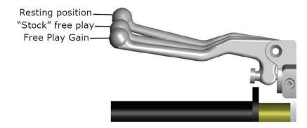
f) When the bike returns to idle, rest your hand across the clutch lever. Rev the engine again to 5,000-7,000 RPM so you can observe the movement while feeling for Free Play Gain with your hand.
