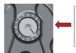
Tick marks are located on the slave cylinder, and an etch mark is on the screw. If you need to re-position the hex key, you can use these marks for reference.
