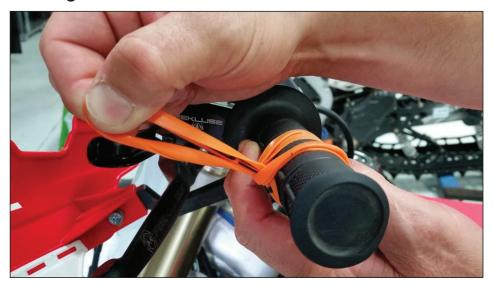
d) Pull the band through the loop, then attach it to the outside end of the clutch lever. This will take up the initial free play (slack) and put the lever in a position to detect the Free Play Gain.
