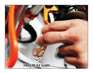
c) While still in **NEUTRAL**, continue to apply light pressure and quickly rev the engine between 5,000-7,000 RPM (1/2 to ¾ throttle), then let it return to idle. Notice the movement in the clutch lever when the engine is revved. This is your Free Play Gain.
