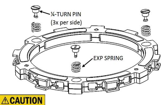
If you disassemble the EXP, the Teflon pads may fall out or be stuck to the ramp surfaces of the EXP bases. Take care to ensure all pads are correctly placed into wedge pockets using gentle pressure to avoid damage to the pad surfaces before reassembling the EXP. Properly seated pads will be secured in place once the EXP is reassembled. Operating the clutch without the pads in place will cause part damage or failure.
