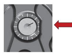
Use the tick marks on the cylinder and the etch mark on the screw to remember the starting point for adjusting the gap.
