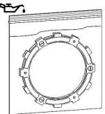
2. Inspect the clutch basket for notching. Do not install sleeves or use product with a notched basket. Notched basket tang faces can cause the sleeves to break. Do not use baskets that have been filed, machined, or modified on the tangs. Replace basket if necessary.
