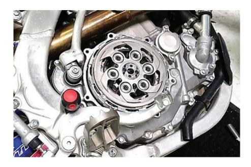
4. Remove the following parts from the clutch. Set aside the old clutch pack. It will not be reused.
