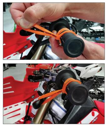
e) While still in NEUTRAL, quickly rev the engine between 5,000-7,000 RPM (1/2 to <sup>3</sup>/<sub>4</sub> throttle), then let it return to idle. Notice the movement in the clutch lever when the engine is revved. This is your Free Play Gain.
