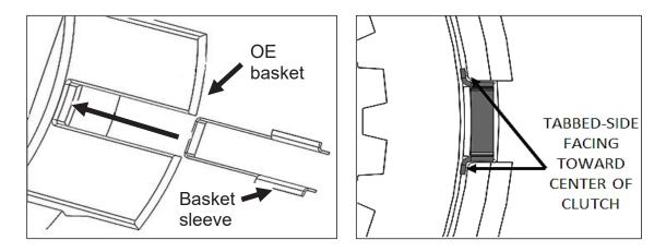
**Note:** When seated in the basket, the sleeves may stick slightly above or below flush with the top of the basket. This is normal.
