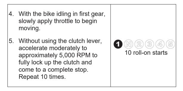
**Note:** If the engine wants to stall or the creep is excessive, the idle may be too high or the installed gap may be too small. Make necessary adjustments before proceeding.
