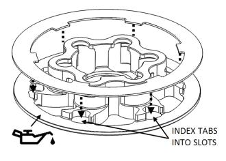
3. Install the pressure plate subassembly.
