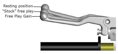
f) When the bike returns to idle, rest your hand across the clutch lever. Rev the engine again to 5,000-7,000 RPM so you can observe the movement while feeling for Free Play Gain with your hand.
