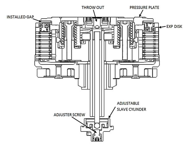
The installed gap is what allows the auto function of the product to perform properly. Setup, break-in, and rechecking the installed gap is **CRUCIAL**. Failure to properly maintain your installed gap can result in premature wear or failure of your clutch.
