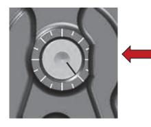
Tick marks are located on the slave cylinder, and an etch mark is on the screw. If you need to re-position the hex key, you can use these marks for reference.
