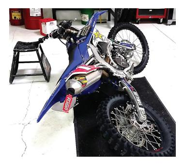
3. Use an 8 mm socket to remove the clutch cover.
