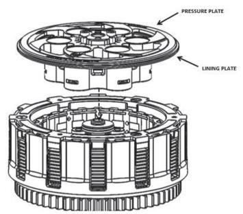
4. Place the pressure plate springs into the assembled clutch, then insert the screw sleeves into the springs. See the following chart for spring information.
