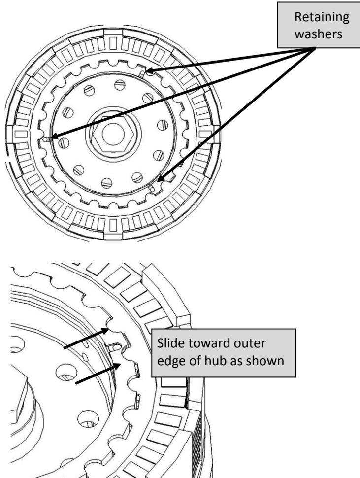
11. Re-install Rekluse lower assembly according to z-Start Pro Manual. It will not install unless the Belleville washers are seated all the way out.
