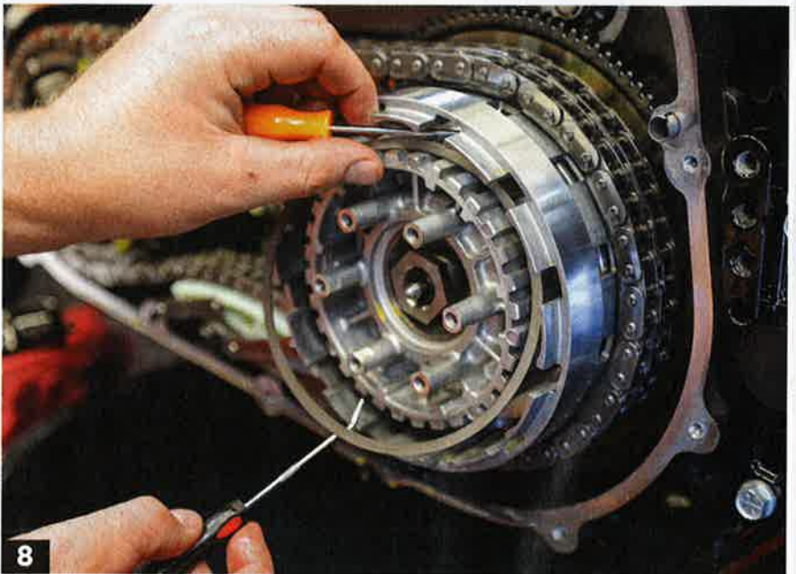
8 ▲ Remove the clutch pack, including the metal judder spring and spring seat. It might be helpful to use picks to remove them.
