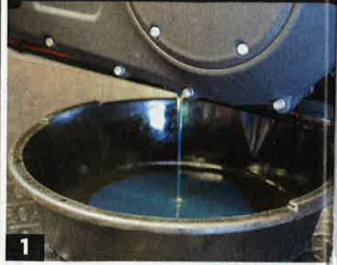
1 ▲ Put the bike on a stand and drain the primary oil.
