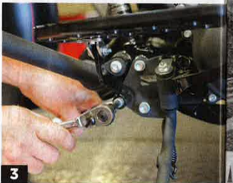
3 ▲ The front shift mechanism and floorboard will need to either be removed or placed out of the way to access the primary cover.
