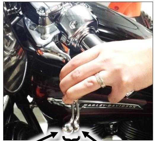
Lever with "slack" removed      Lever position around 4,000 RPM
