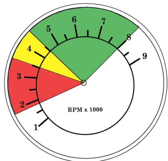
4,500 RPM. The clutch is fully clamped at this point. Any technical trail riding or ascending a grade should be done in this range. Upshift and downshift as you normally would using the clutch lever.
