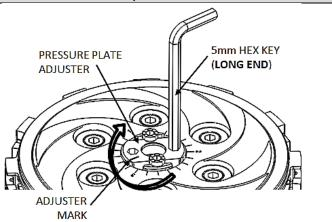
10. At this point, make a note of where the mark on the adjuster aligns with the tick marks on the pressure plate. This is your **starting point.**
