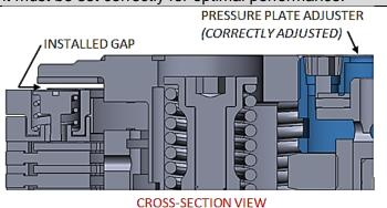
9. Insert the **long end** of a 5-mm hex key into one of the two hex holes in the pressure plate adjuster. By hand, **gently** thread the pressure plate adjuster inward until it comes to a stop against the center clutch nut.
