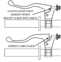
**NOTE:** The pressure plate adjuster should bottom out and lift against the center clutch nut, not the throw-out. Slack in the clutch cable ensures that you find the correct starting point.
