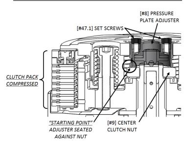
12. Now, insert the **short end** of the 5-mm hex key into the pressure plate adjuster, and turn it clockwise **one full turn plus 2 tick marks past the starting point** (aka "1+2").
