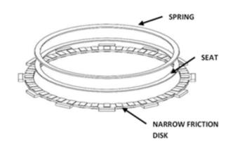
• If judder spring and seat are installed, assemble the clutch following the graphic on the next page. .
