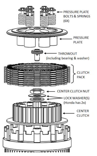
**Note:** Some models come equipped with a judder spring seat and judder spring. These are typically found at the bottom of the clutch pack inside a narrower friction disk. Be sure to remove these parts with the clutch pack.
