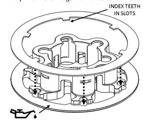
7. Install this pressure plate subassembly.
