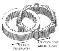
Inspect the friction disks for signs of heat or wear. Replace if they are burnt or worn. For most models, new friction disks can be purchased from Rekluse.
