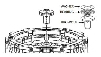
**NOTE**: If you are missing the top washer, it is probably stuck to the backside of your OEM pressure plate.
