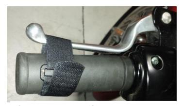
Clutch Lever Strap: to prevent unwanted launching.
